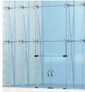
TENSION ROD STRUCTURE
